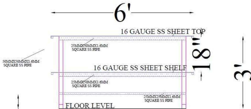
7" SECTION OF SS STORAGE UNIT SIZE (6'X2'6")
